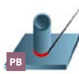
PB Teava: fixa Axa: verticala Sudura: orizontala
